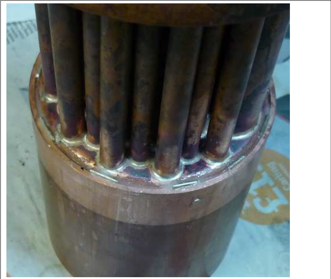
Bottom tubeplate soldered and ready to solder into inner firebox
