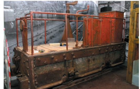
Baldwin-built, 2ft 6in gauge electric locomotive of 1902. HUGH DOUGHERTY
